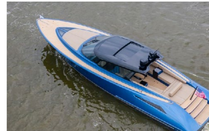
Roof design for extra large glass and composite panels
